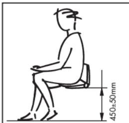
Determine the height of the seat. A distance of 45 cm is recommended from either bathroom floor, or floor of the shower tray, to the underside of the seat when hinged down (equivalent to 55 cm from the lower edge of the mounting plate). For personal preference the seat can be situated higher or lower according to your body height.
