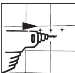
Drill the marked holes with a 8 mm diameter masonry drill to a minimum of 80 mm.
