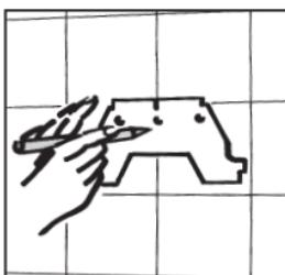
Fix the mounting plate horizontally at the required height. Mark the positions of the 3 fixing drillings by using the mounting plate as a drilling template. Be sure that there are no water pipes or electrical wiring behind the location you intend to fix the seat to.
